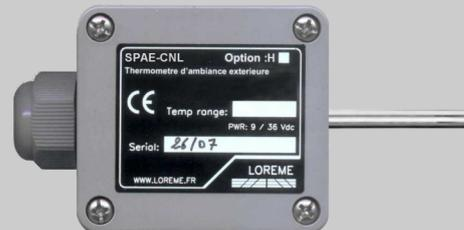
These probes allow to measure the ambient temperature in a room and provide a 4-20 mA loop powered output signal. The measure element (Pt 100 platinum RTD probe) used ensures an excellent repeatability of the measures.
