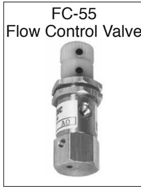
These precision machined valves are designed and manufactured to provide Micro-Fine™ control of gasses and liquids. They have a micrometer pitch (40 threads per inch) adjusting thread and precision machined tapered needle and seat. They are available as needle valves and flow control valves.
