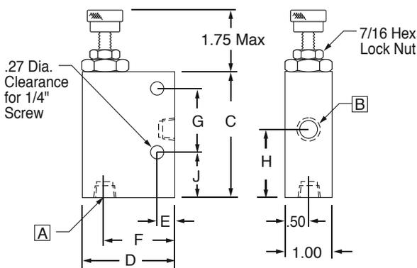
Super-Vee™ Flow Control controls one direction – Free flow return
