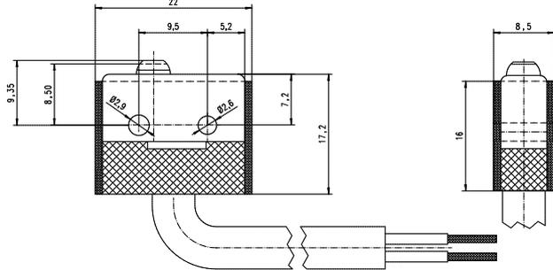
**Response monitoring microswitch – KZ** – control of the state of brake (engaged, disengaged),
