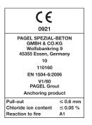
According to the 3rd correction of DAfStb Rili SIB (8) may V1/50 PAGEL-GROUT and V1/160 PAGEL-GROUT (both SKVB I and early strength class A) be used for reprofiling concrete structures such as concrete after DIN EN 206-1 in conjunction with DIN 1045-2 (maximum permissible Layer thickness 100 mm).
