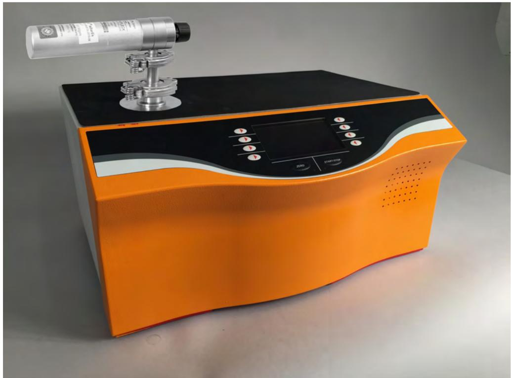
Fig. 15: Checking an external calibration leak
