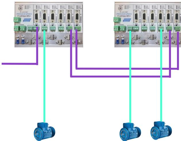
Fig. 17 - Redundant path between two ProfiHubs
