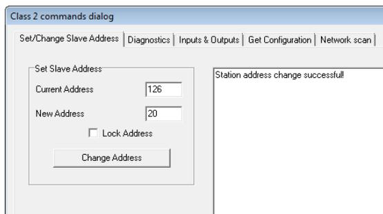
Fig. 21 - ProfiCaptain changes the address from 126 to 20
