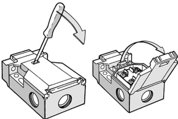
Access the wiring chamber via a hinged door. Simply insert a flat-blade screwdriver, as shown, and pry gently down to open.
