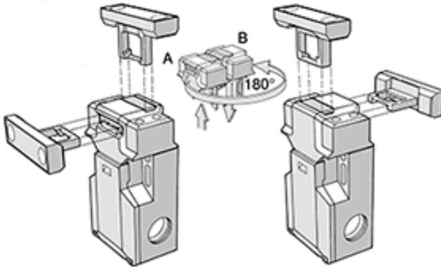
The actuator head may be rotated 180° to create four possible actuator engagement locations. To rotate the head:
