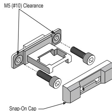
1. Temporarily mount the switch body in place, with its actuator inserted, using the slotted 5 mm holes. The slotted holes in the switch body must **ONLY** be used for alignment during installation. The round 5 mm holes (only) must be used for permanent mounting to prevent loosening or displacement of the actuator and the switch body. Only M5 (#10) screws (user supplied), should be used.
